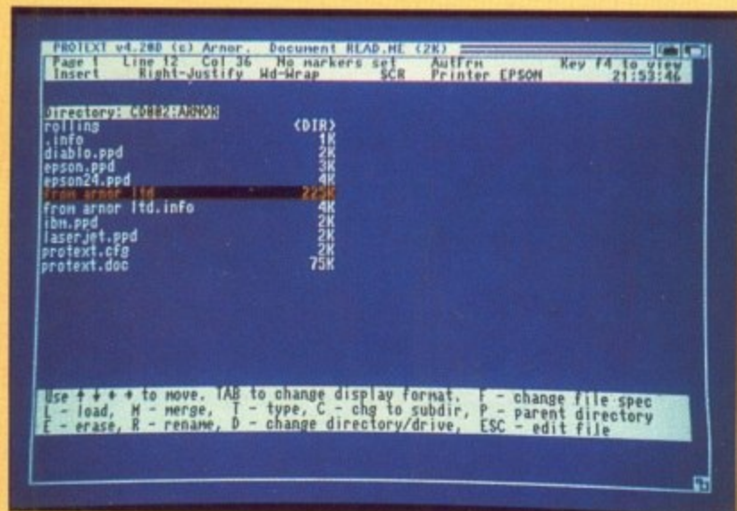
The File Manager option is reached by pressing Right-Amiga-C in Edit mode or choosing Catalogue from the Project menu.
